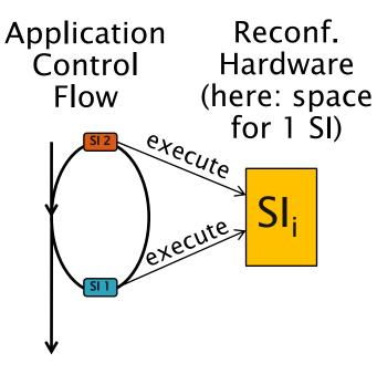
→ two reconfigurations <u>per</u> <u>loop iteration</u>, i.e. configuration thrashing
